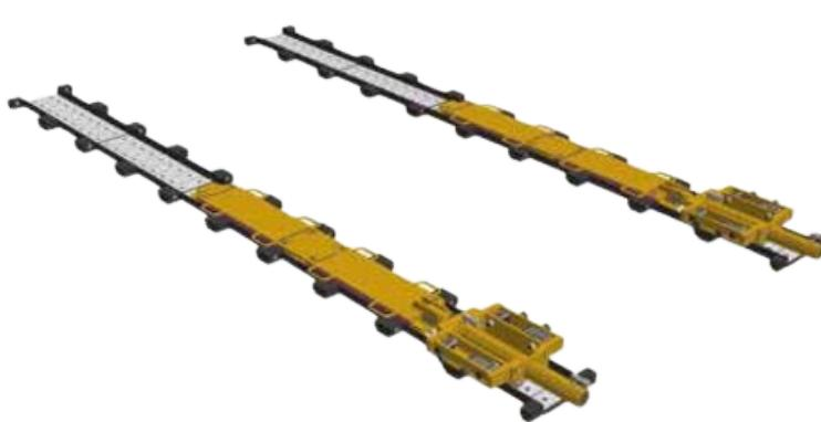
Our Low Height Skidding System is a modular system that can jack and slide heavy loads over a pre-constructed track. The Low-Height Skidding System is comprised of a series of skid beams moved by hydraulic push-pull units, travelling over a pre-constructed track. A series of special PTFE-coated pads are placed on the skid tracks to reduce friction. The push-pull units are powered by a standard Enerpac Split Flow Pump (ordered separately) to ensure each skid beam travels synchronously.
