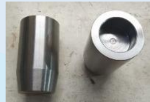
Figure 2: CNC machining of a spare part for integration in structural repairs
